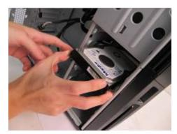
Caution: Do not torque or over-tighten the 3.5" internal drive tray screws. Compressing the silicone grommets will reduce their lifespan and will lessen or negate their vibration-insulating effect. Tighten the screws until you feel resistance, then STOP.
